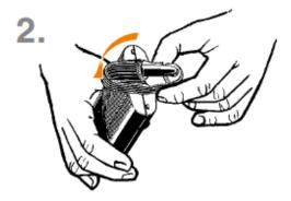
Removal of Cooling Unit (with Mouthpiece)
